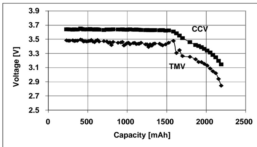
Figure 3: AA size Li/SOCl<sub>2</sub> and HLC-14500 battery pack discharged at pulses of 500mA 1sec once per week (average current - 110μA).
