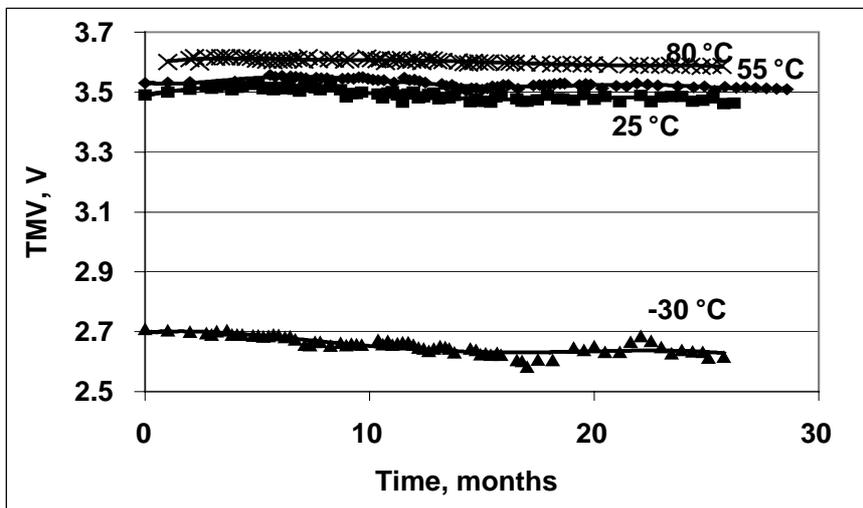
Figure 5: Minimum voltage under 500mA sec. pulse for AA size Li-SOCl<sub>2</sub>+ HLC-14500
