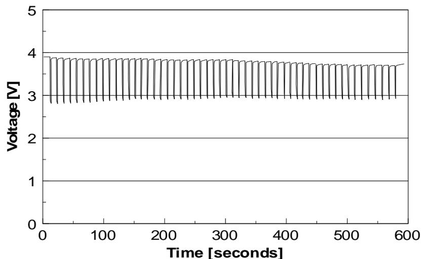
Figure 2: 10A 1 sec pulses every 10 sec. to AA size  $\text{Li-SO}_2\text{Cl}_2$  and HLC-14500 at RT.
