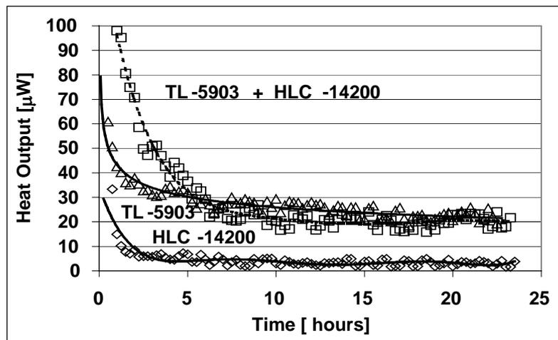
Figure 7. Microcalorimetric measurement under OCV conditions of Pulses Plus battery comprising of AA Li/SOCl<sub>2</sub> cell and HLC-14200 after 8 months at RT
