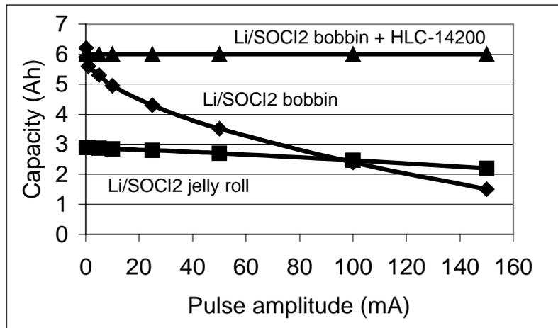
Figure 8. Available capacity to 2.5 V cut off versus current amplitude for C-size cells under 5 sec pulse at RT (average current –  $70\mu\text{A}$ )
