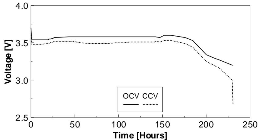
Figure 6: OCV and the minimum voltage during 1.4sec 350mA every 5 seconds pulses at 125°C of DD size Li/SOCl<sub>2</sub> and HLC-14200.
