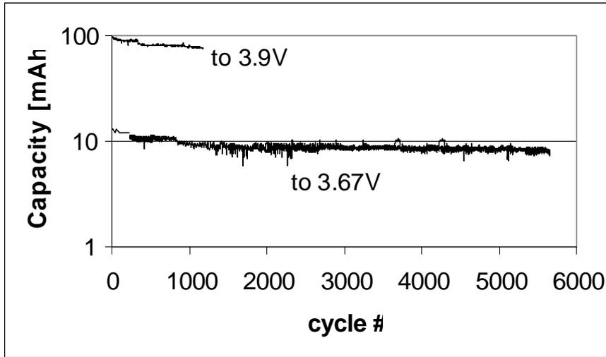
Figure 4: Discharge capacity vs. cycle # to 3.67V and to 3.9V of HLC-14200
