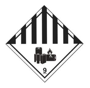
Class 9(A) Hazard Label for lithium batteries
