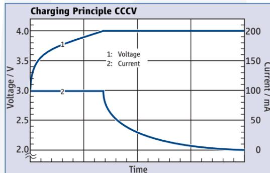
Figure 1: Charging principle CCCV. Example for TLI-1550
