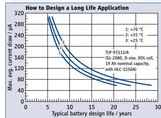
Figure 3: How to Design a Long Life Application
