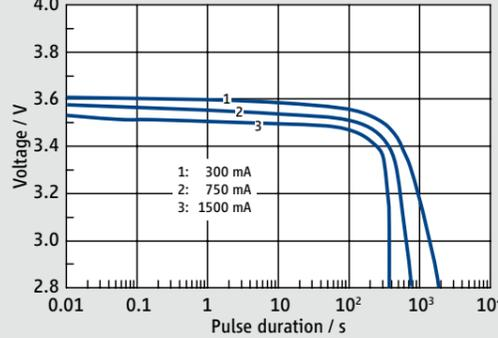
**Maximum Pulse Width from 3.6 V to 2.8 V**
