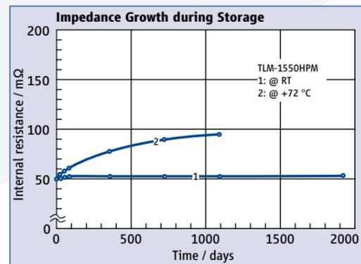
Figure 3: Impedance Growth during Storage
