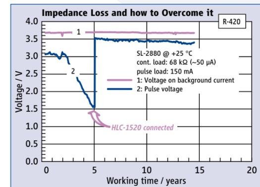
Figure 1: Impedance Loss and how to Overcome it
