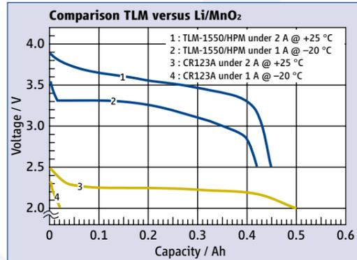
Figure 1: Comparison TLM versus Li/MnO<sub>2</sub>
