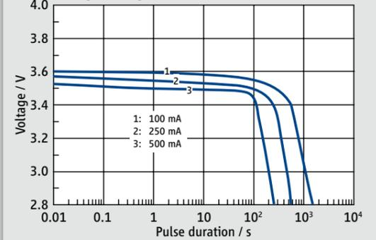
**Maximum Pulse Width from 3.6 V to 2.8 V**
