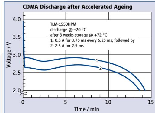
Figure 2: CDMA Discharge after Accelerated Ageing
