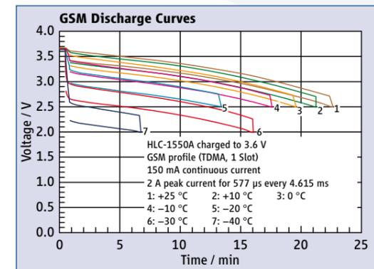
Figure 2: GSM Discharge Curves
