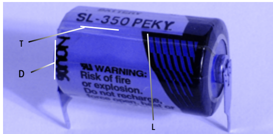
Figure 6-3 Battery with type number (T), lot number (L), and date (D) of final inspection. Inquiries should make reference to the lot number.
